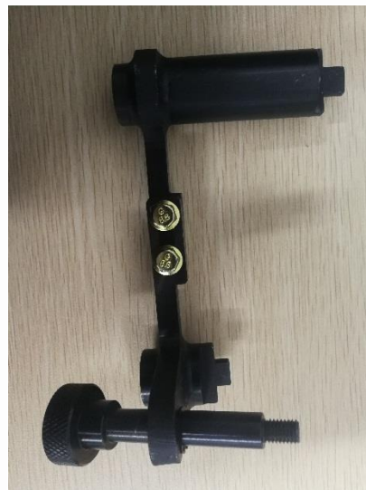
Camshaft fixing tool
