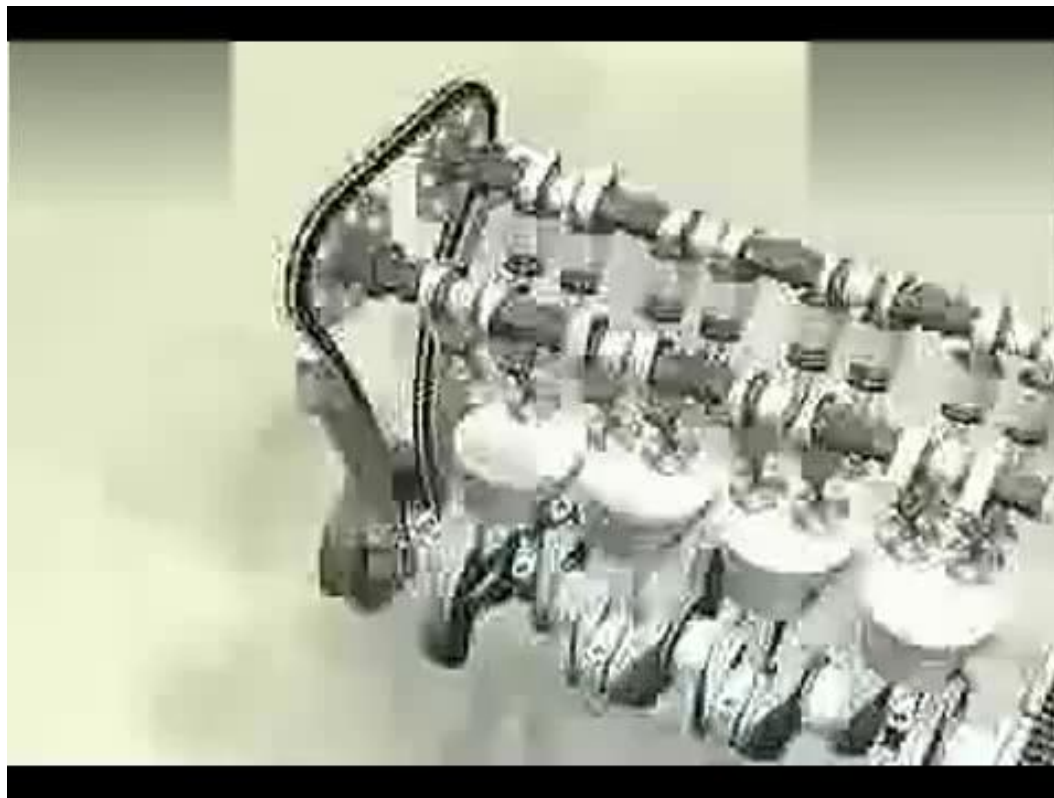
Crank connecting rod mechanism
